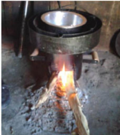
Recent tests of the Jiko Poa cookstove confirmed its fuel efficiency and indicated significant indoor air pollutant reductions compared with traditional cookstoves.
